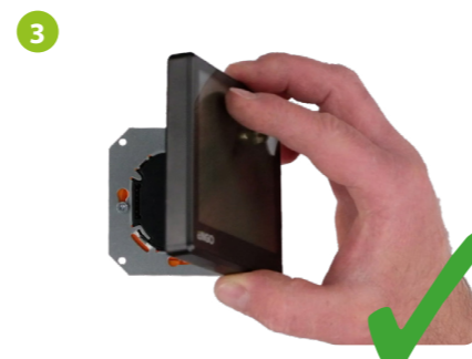
Slide the front of the controller over the back part. Turn on the power supply. The controller is ready for operation.
