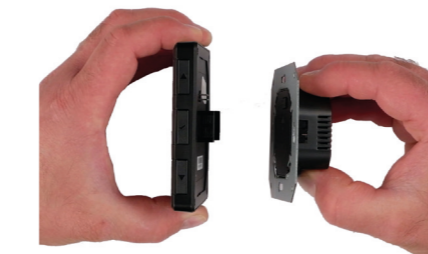
Grab the top part and the bottom part to disconnect
