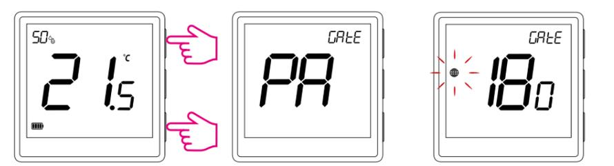
Make sure ZigBee Gateway has been added to the Engo Smart app. Press and hold the ▲ and ▼ buttons on the thermostat until the display shows „PA”. Then release the keys. The pairing mode will be started up.
