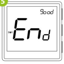
After successfull binding operation „End“ message will be displayed. LED on the module will stop flashing.
