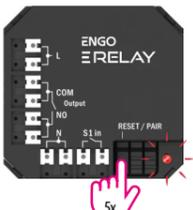
To properly link thermostat with the module/relay first click quickly the button on the device 5 times. The LED diode will start flashing slowly on red, which means the device is in binding mode.
