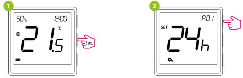
Use ▲ or ▼ . button to move between parameters. Enter the parameter by ✓ . Edit the parameter using ▲ or ▼ . Confirm the new parameter value with the ✓ button.
