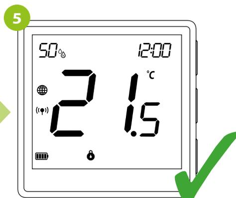
When the buttons are locked, only the currently measured temperature can be read on the thermostat.
