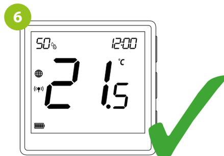
Both devices have been successfully linked. Thermostat displays the main screen, icon (☺) appeared on the screen indicating connection with the receiver.
