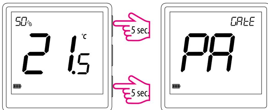
On the EONE thermostat, hold ▲ and ▼ buttons simultaneously for 5 seconds until „PA” appears on the display. The thermostat will enter pairing mode.
