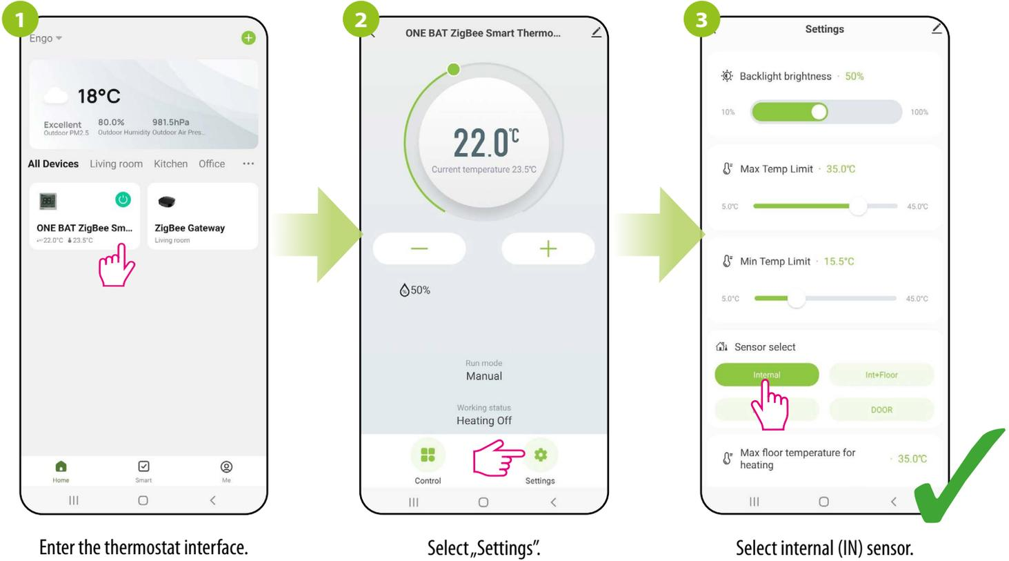
**Internal sensor + floor temperature sensor** - if you connect an additional floor sensor to terminals S1/S2 of the thermostat, both sensors are active (internal and external). The internal sensor measures and controls the room temperature, and the additional sensor acts as a protection of the floor against overheating and overcooling.
