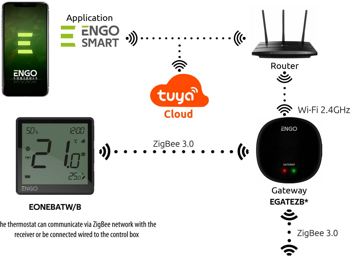
The thermostat can communicate via ZigBee network with the receiver or be connected wired to the control box
