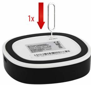
On the EGATEZB gateway, press the RESET button. The green LED will start flashing. Pairing mode will then be invoked.
