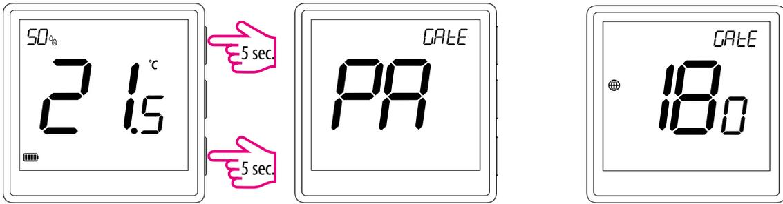
On the EONE thermostat, hold ▲ and ▼ buttons simultaneously for 5 seconds until „PA” appears on the display. The thermostat will enter pairing mode and count backwards (180s).
