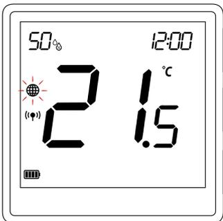
**(GLOBE ICON) is flashing** – Connection to ZigBee gateway is lost.
