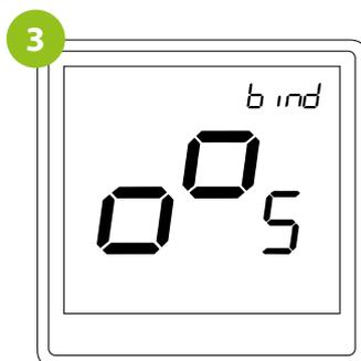
Release keys, binding function is active.
