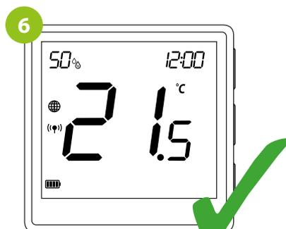
Both devices have been successfully linked. Thermostat displays the main screen, icon "((⬆))" appeared on the screen indicating connection with the receiver
