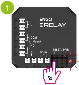
To properly bind thermostat with the relay first click quickly the button on the device 5 times. The LED diode will start flashing slowly on red, which means the device will enable binding mode.
