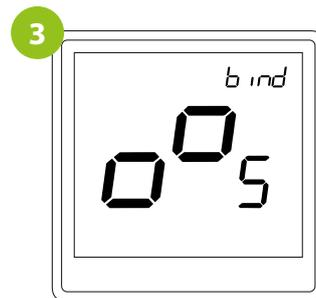
Release the keys, binding function (process of linking thermostat) is active.
