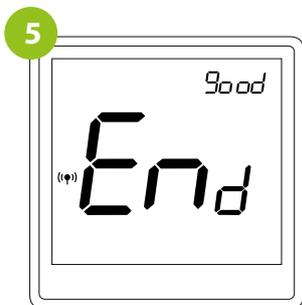
After successful binding operation „End” message will be displayed. LED on the module will stop flashing.
