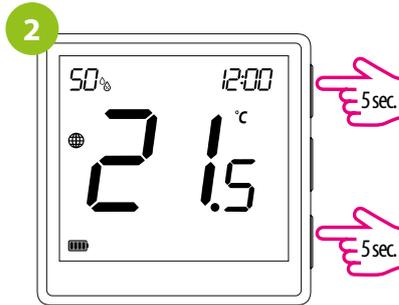
On the EONE thermostat, hold ▲ and ▼ buttons at the same time for 10 seconds until the „bind” function appears.
