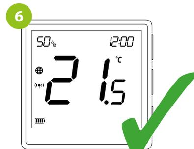
Both devices have been successfully linked. Thermostat displays the main screen, icon (📶) appeared on the screen indicating connection with the receiver.
