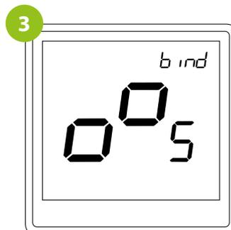
Release keys, binding function is active.
