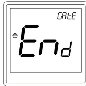
After the pairing is completed, the thermostat show End message on the display.
