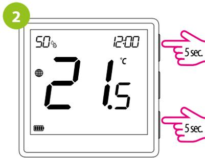
On the EONE thermostat, hold and buttons ▲ and ▼ for 10 at the same time seconds until the „bind” function appears.
