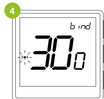
The "binding" process takes up to 300 seconds.
