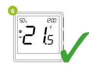
Both devices have been successfully linked. Thermostat displays the main screen, icon " ((♠)) " appeared on the screen indicating connection with the receiver (module/relay in this case).
