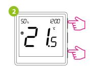
On the EONE thermostat, hold **a** and **v** buttons until the "bind" message appears.
