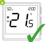
Both devices have been successfully linked. Thermostat displays the main screen, icon " (( •)) " appeared on the screen indicating connection with the receiver (ECB62ZB in this case).
