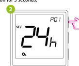
Use ▲ or ▼. button to move between parameters. Enter the parameter by ✓. Edit the parameter using ▲ or ▼. Confirm the new parameter value with the ✓ button.
