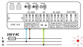
Power supply for wiring centre is  $230 \text{ V} \sim 50 \text{Hz}$ .
