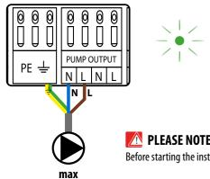
When the Pump/Valve control output is activated, the pump status LED shows a constant green light.
