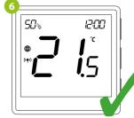
Both devices have been successfully linked. Thermostat displays the main screen, icon " $((\mathbf{r}))$ " appeared on the screen indicating connection with the receiver (ECB62ZB in this case).
