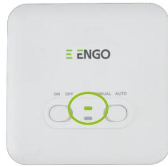
When the green diode on the receiver lights up continuously, the devices have been paired on a new frequency.
