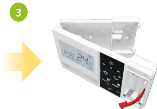
Separate the front part from the back part in the direction shown above.
