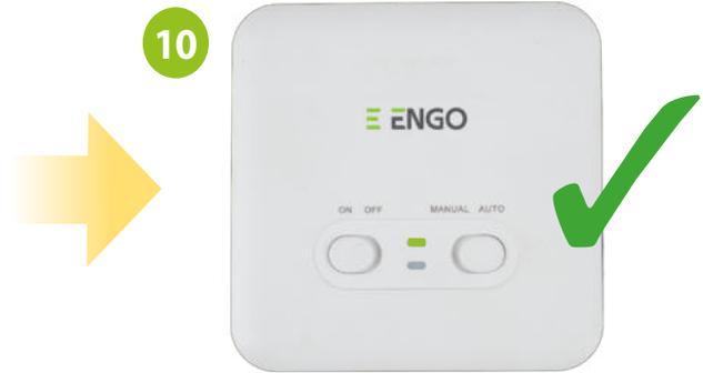
...and the orange LED on the receiver should go out.
