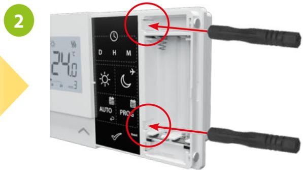
Use a screwdriver to push the plastic tabs in as shown in the figure until you feel resistance, and tilt the front part of the housing.
