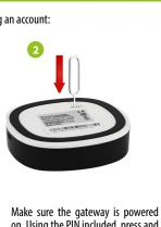
non. Using the PIN included, press and hold the RESET button for 8 seconds until LEDs start lighting up. The pairing mode is enabled.
